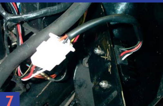
7 CONNECT THE BLOCK CONNECTOR TO THE IGNITER BOX AND WIRE UP AS THE DIAGRAM SPECIFIES FOR YOUR MOTORCYCLE (+ OR - EARTH ETC).
